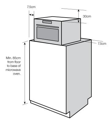
Blocking the intake or outlet vents can damage the oven. If air vents are blocked during operation, the oven may overheat, and this may lead to malfunctioning. Hot air escapes from the vents, so be sure not to obstruct it or let curtains come between the oven and the rear wall.
