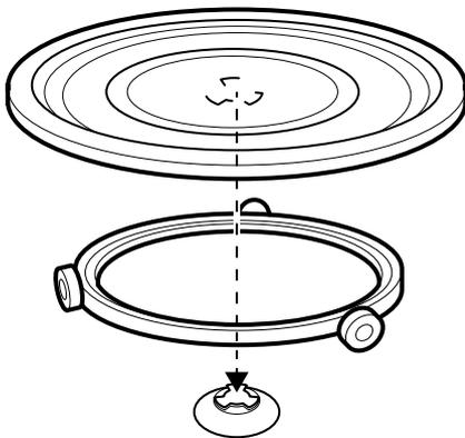
1. Place the roller guide around the turntable shaft.
