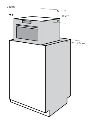
Blocking the intake or outlet vents can damage the oven. If air vents are blocked during operation, the oven may overheat, and this may lead to malfunctioning. Hot air escapes from the vents, so be sure not to obstruct it or let curtains come between the oven and the rear wall.
