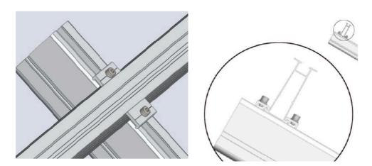
Clamp the cross members to the uprights using the GS-8R-C60 clamps (2 per rail i.e. clamp from both sides. Tighten to 10Nm.
