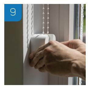
Attach the Smart Shades to the wall. Use the tape on the back of the device or screws (not included). Make sure that the chain is not crossed or too loose/tight. See the following images.
