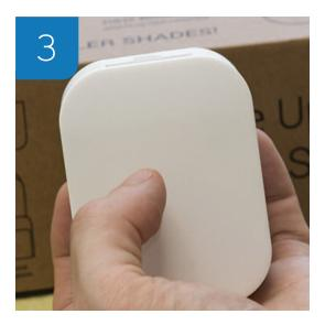
Hold your hand on the front panel for few seconds to activate Smart Shades. The Device has a touch sensitive front panel.
