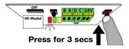
3. On the new remote, press and hold any button (should only take about 1-2 seconds) that you wish to operate the door. The LED on the motor should stop flashing once the remote has been programmed.
