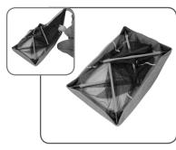
7a. To fold the **Frame**, slightly lift the frame on one end and press the large release buttons beneath the fabric on the inside of the **Top Frame** on both sides.
