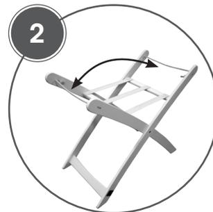
2a. Spread the legs in order to unfold the stand.
